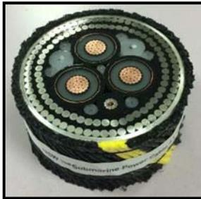
**Fig. 1: 3x150 mm<sup>2</sup> copper 20 kV XLPE Submarine cable**
