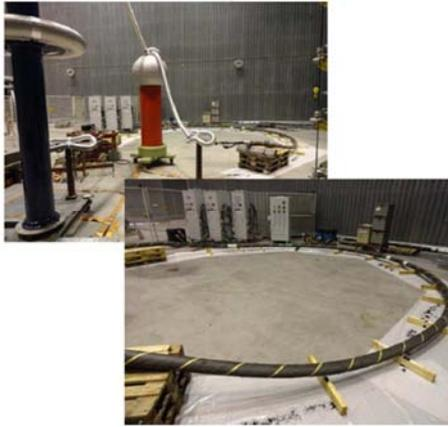
**Fig. 3: Electrical type tests set up**
