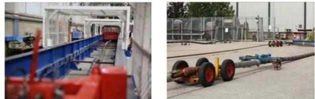
**Fig. 3: Traction and Tensile bending test on 3x150 mm<sup>2</sup> copper MV XLPE Submarine cable**
