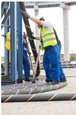
**Fig. 2: Coiling test on 3x150 mm<sup>2</sup> copper MV XLPE Submarine cable**
