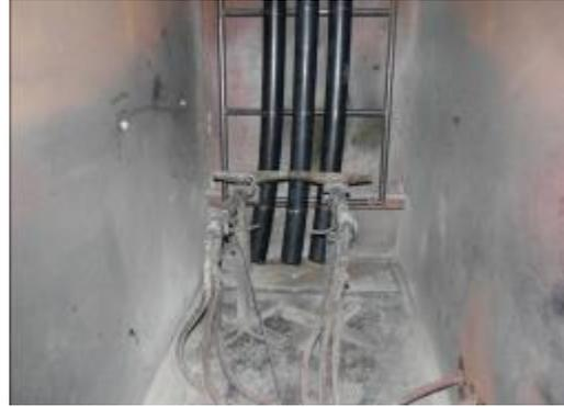
(5) Non-fire spread test category A, with special assembly of a triad of cables in trefoil formation, on 300 mm ladder and one burner, with three clamps KOZ TRI 3x without metal protection (separation between clamps 120 cm; first clamp at 25 cm from the burner):
