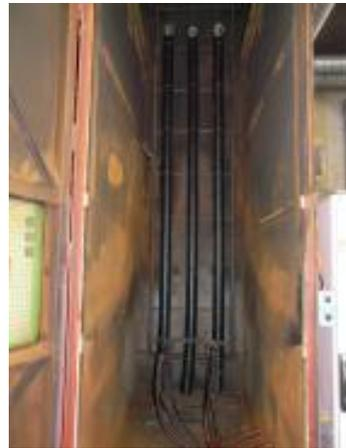
(7) Non-fire spread test category A, with special assembly of two pieces of cable, separated the maximum distance between them (300 mm approx.),
