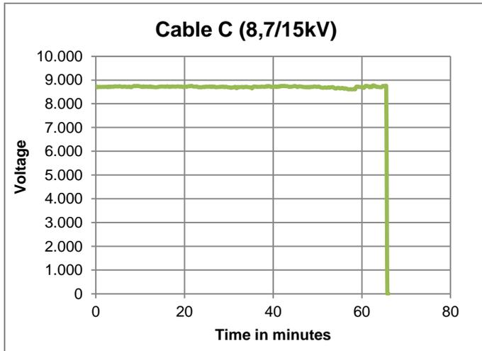
Figure 5 – Test results and time to breakdown
