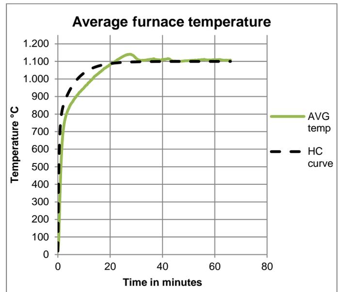
Figure 2 – Average furnace temperature
