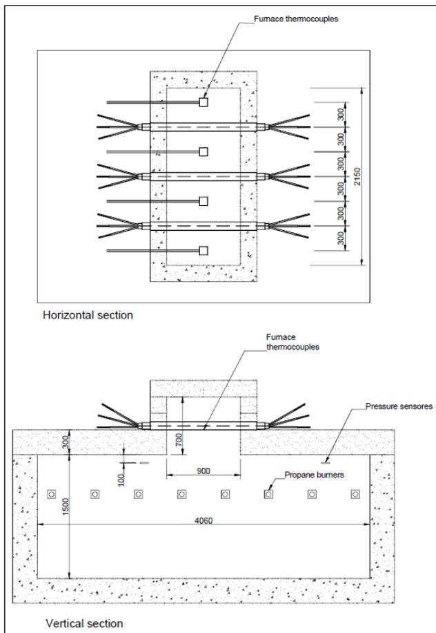
Figure 1 – Furnace setup
