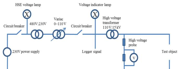
Figure 4 – Electrical circuit
