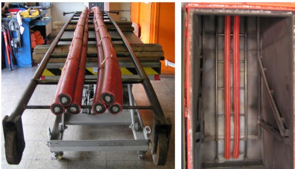
**Figure 1: Cables on the stairs forming two triads**
