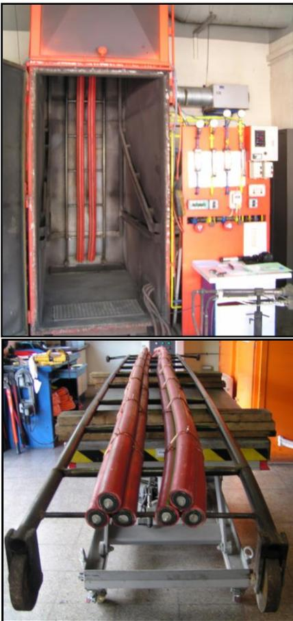
**Figure 7: Cables on the stairs forming two triads**
