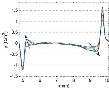
**Figure 8: Evolution of space charge density during poling at -80 kV for 90 min in the case of a full HVDC commercial formulation XLPE model cable.**
