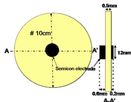
Figure 1: Typical geometry of plaque samples.
