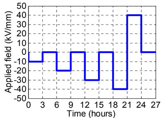
**Figure 3: Stress cycle applied for space charge measurements on flat specimens.**
