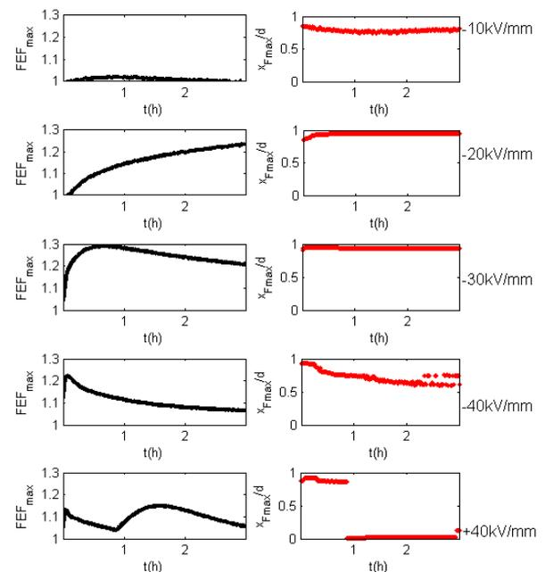
**Figure 5: Evolution of the  $FEF_{max}$  and its position vs. time under various fields for the gold-metalized HVAC-XLPE sample.  $x=0$  (d) for anode (cathode).**
