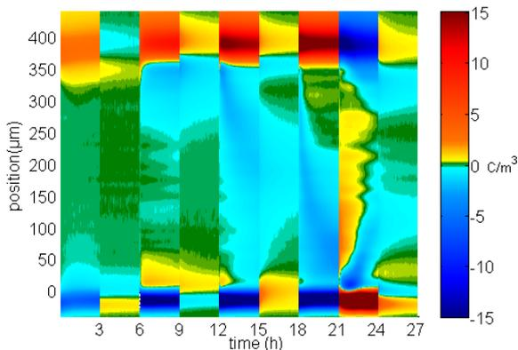
**Figure 4: Space charge pattern for a gold-metalized HVAC-XLPE sample obtained using the protocol of Figure 3.**
