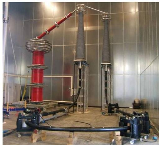
Fig. 13: Type test set-up of the 320 kV cable systems
