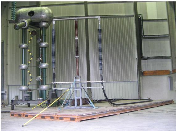
Fig. 12: Type test set-up for 270 kV LCC cable systems
