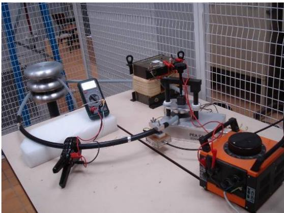
**Fig.3: Test bench up to 100kV DC for cable model**
