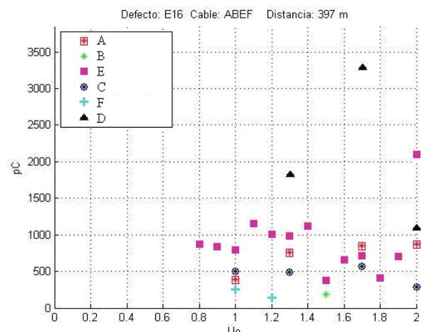
**Fig. 4 PD activity on a joint.**
