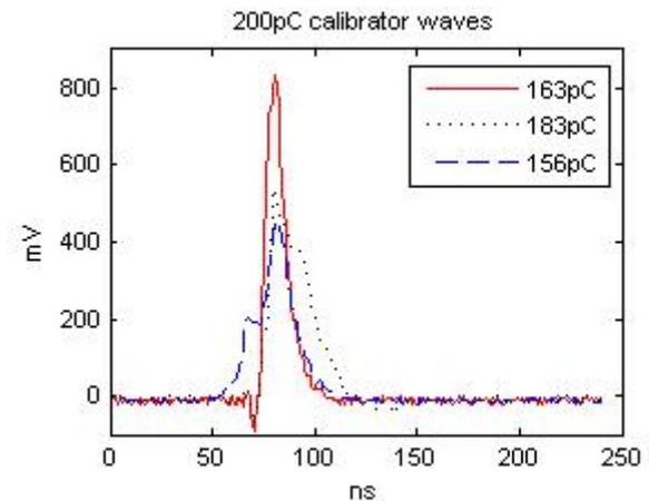
**Fig. 3 Pulses of 200pC of three different calibrators.**
