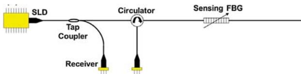
Fig 3: Measuring scheme
