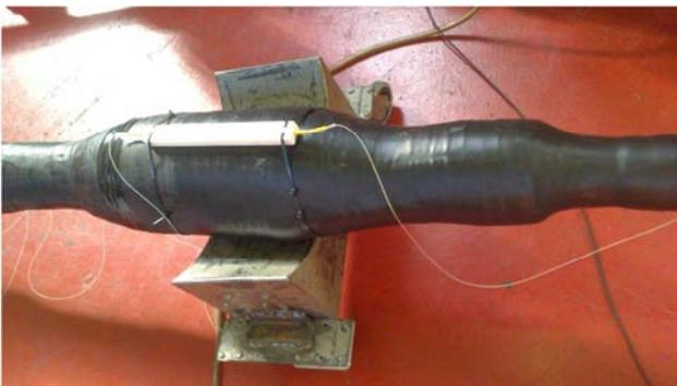
Fig 7: LTS sensor installed on a joint
