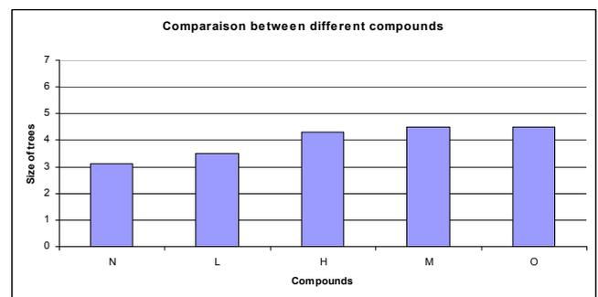
**Figure 6: impact of the additives on the water-trees size**
