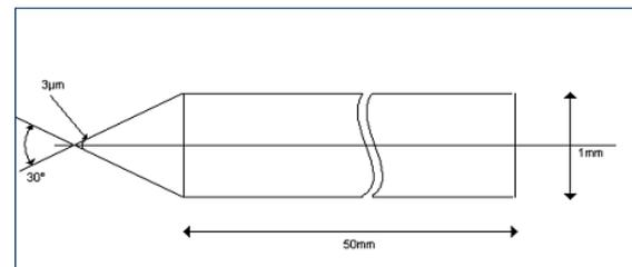
Figure 1: Dimensions of needles
