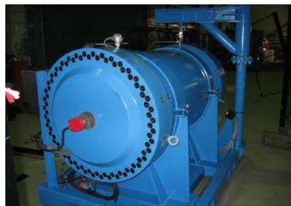
Fig. 2: Pressure vessel used for hyperbaric ageing at General Cable Manlleu Testing Laboratory
