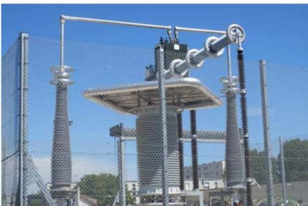
**Fig. 9: 320kV DC outdoor terminations during the prequalification test**
