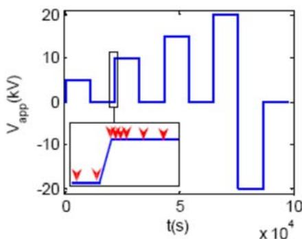
Fig. 2: Applied voltage protocol for a EPDM insulation with a thickness of 600μm and acquisition procedure illustration. Each voltage step lasts for 3h.
