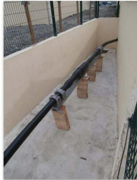
**Fig. 10: 320kV DC underground premoulded joint**
