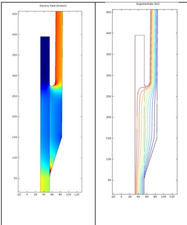
**Fig. 5: Electric field distribution in premoulded joint**
