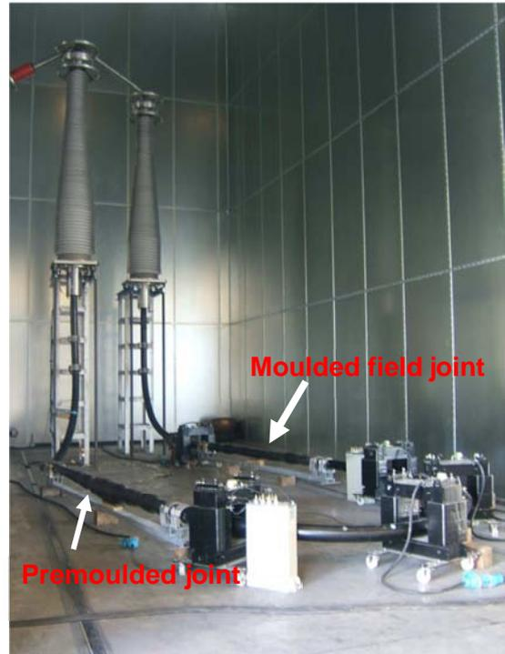
**Fig. 6: Type test set-up of the 320 DC kV cable systems**
