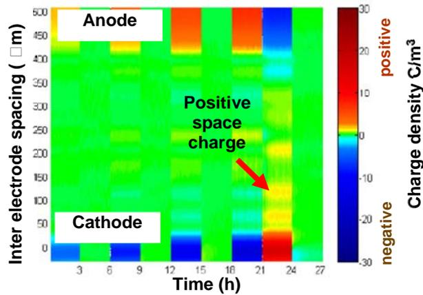
Fig. 3: Spatial distribution of Space charge in plaque of EPDM during the poling and depolarization, respectively
