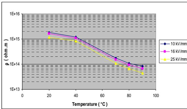
Fig. 1 : DC resistance properties of EPDM
