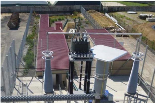
**Fig. 8: 320kV DC prequalification test laboratory**
