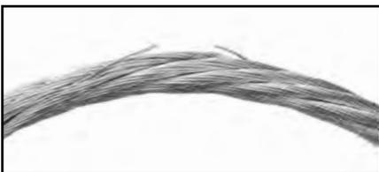
The third sample was again flexed the same number of cycles using the same tension as with the control sample. However, a bending radius two and one-half times larger was used. Increasing the bending radius practically eliminates strand damage.
