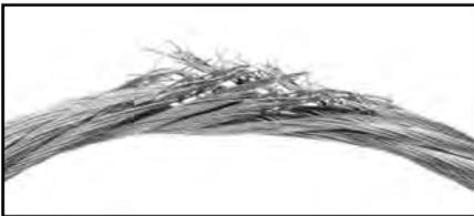
The control sample was flexed continuously for a specified number of cycles over a given bending radius, under specific tension, until only a few strands remained unbroken.
