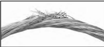
The second sample was flexed the same number of cycles over the same bending radius, but the tension weight was reduced by one half. As can be seen, reduction of tension greatly reduced strand breakage.
