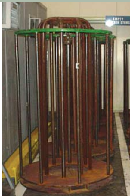
General Cable's Lawrenceburg, Kentucky plant delivers interplant shipments of drawn copper on returnable stem containers.
