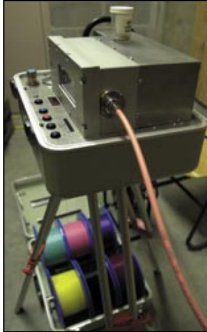
Once the tubes are in place, a two-person crew then uses specialized blowing equipment that delivers clean, compressed air to quickly and easily propel up to 12 optical fibers through each tube.
