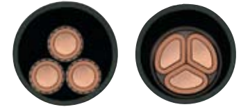
500 kcmil 15K Cable in 3" Duct
